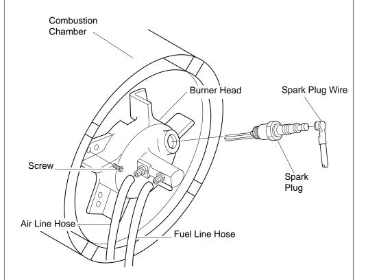
Figure 14 - Removing Burner Head, 100,000 BTU/Hr Model
